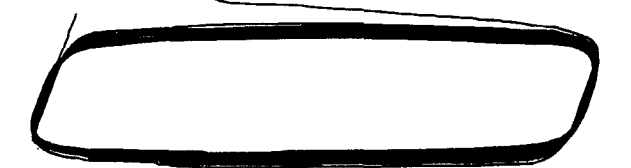
Figure 8—Effect of storage on stress/strain hysteresis loop for white soft paraffin, nonlinear testing, n = 5 \times 10^{-3} Hz. Strain amplitude = 2.0 \times 10^{-2} rad. Gap = 6.4 \times 10^{-2} cm.
